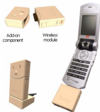
Fig. 1. Buoy: wireless advertising and discovery device
